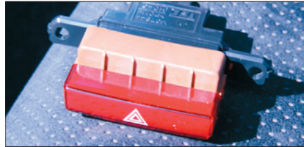
16. uninstall hazard light switch
