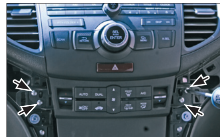
7. Remove screws of air condition control unit
